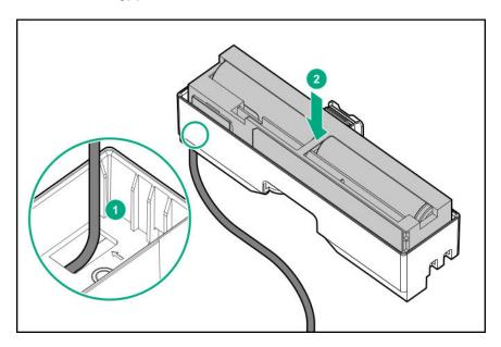
**10.** Secure the energy pack cable through the holder cable clips.
