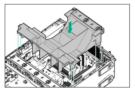
2. Press down the air baffle and make sure that the tabs on the blue latches are engaged in their chassis slots.
