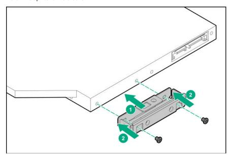
**11.** Install the optical drive in the drive cage.
