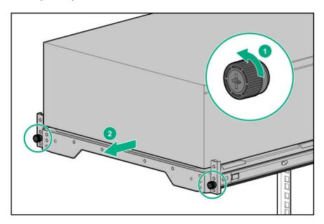
WARNING: To reduce the risk of personal injury, be careful when pressing the server rail-release latches and sliding the server into the rack. The sliding rails could pinch your fingers.
