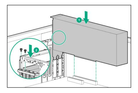
**15.** Make sure that the board is firmly seated in the slot.
