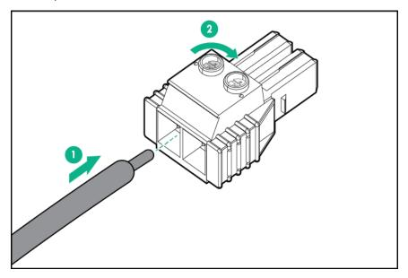
Insert the return wire into the right side of the connector, and then tighten the screw to  $1.3~\mathrm{N}~\mathrm{m}$  (10 lb-in) of torque.
