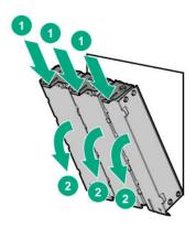
If the drive cage is to be installed in box 2 or 3, remove the drive cage blank. Retain the blank for future use.
