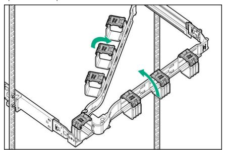
Route the rear panel cables and power cords though the CMA, and then close the cable clamps. Employ industry best practices in routing and managing these rear panel cables and power cords.
