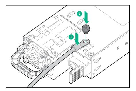
**7.** Insert the -48 V wire into the left side of the terminal block connector, and then tighten the screw to  $1.3~\mathrm{N}~\mathrm{m}$  (10 lbin) of torque.
