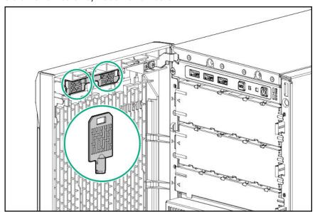
• Hang the front bezel key from the padlock eye on the rear panel.
