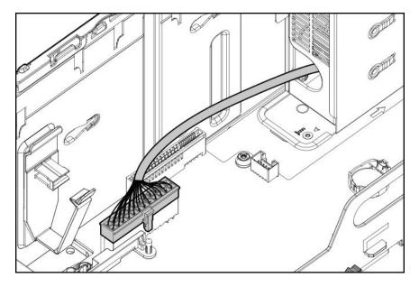
**12.** Remove the non-hot-plug power supply.
