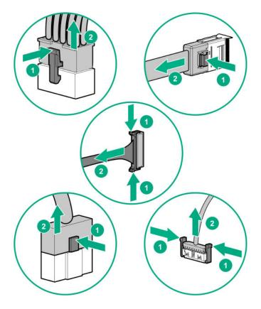
• Remove cables that are no longer being used. Retaining them inside the server can restrict airflow. If you intend to use the removed cables later, label and store them for future use.
