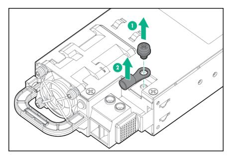
**3.** Crimp the ring tongue to the ground cable from the -48 V DC power source.
