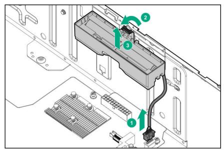
**11.** Disconnect the non-hot-plug power supply cable.
