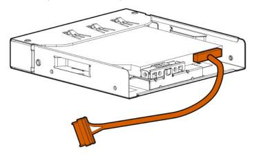
**14.** Slide the optical drive assembly with the SATA-power cable into the optical drive bay until it clicks into place.
